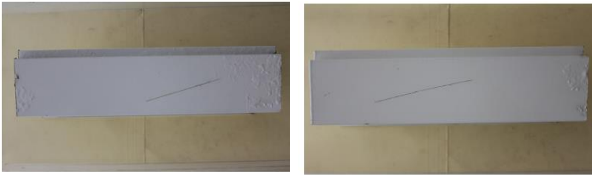
Figure 3. Corrosion on covered (left) and non-covered (right) parts in AAMA weathering tests
